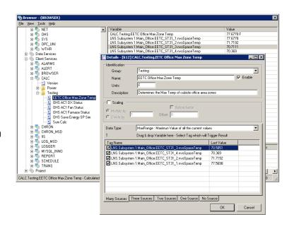
The calculator service runs within the Opendiem Engine. Calculated tags can be viewed using the Opendiem Engine Browser, trended in the data logger, monitored with the alarm manager, used as variables in additional calculations, and displayed on graphical web screens or WBC reports.
